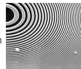
Zone plate x-ray "lens" Outer ring spacing ~35 nm
